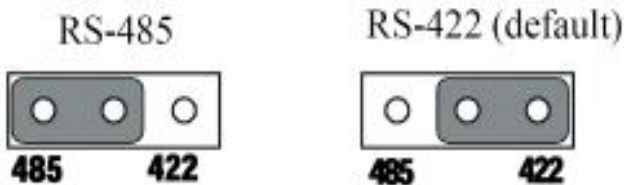
Figure 2.22: RS-422/485 Selection by Jumper Setting
