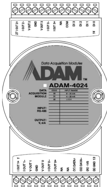
Figure 3-38 ADAM-4024 4-channel Analog Output Module
