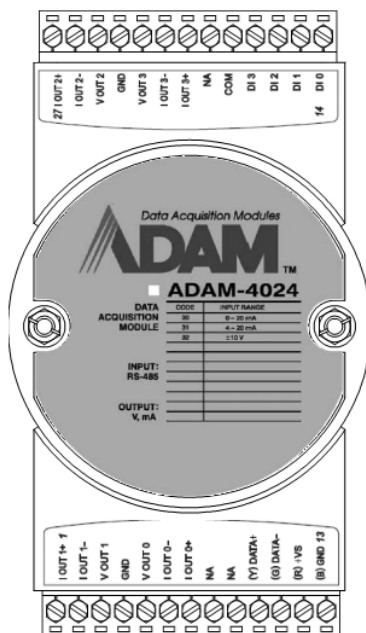
Figure 3-38 ADAM-4024 4-channel Analog Output Module
